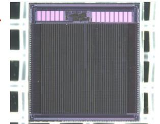
Low-dropout Regulator ASIC
