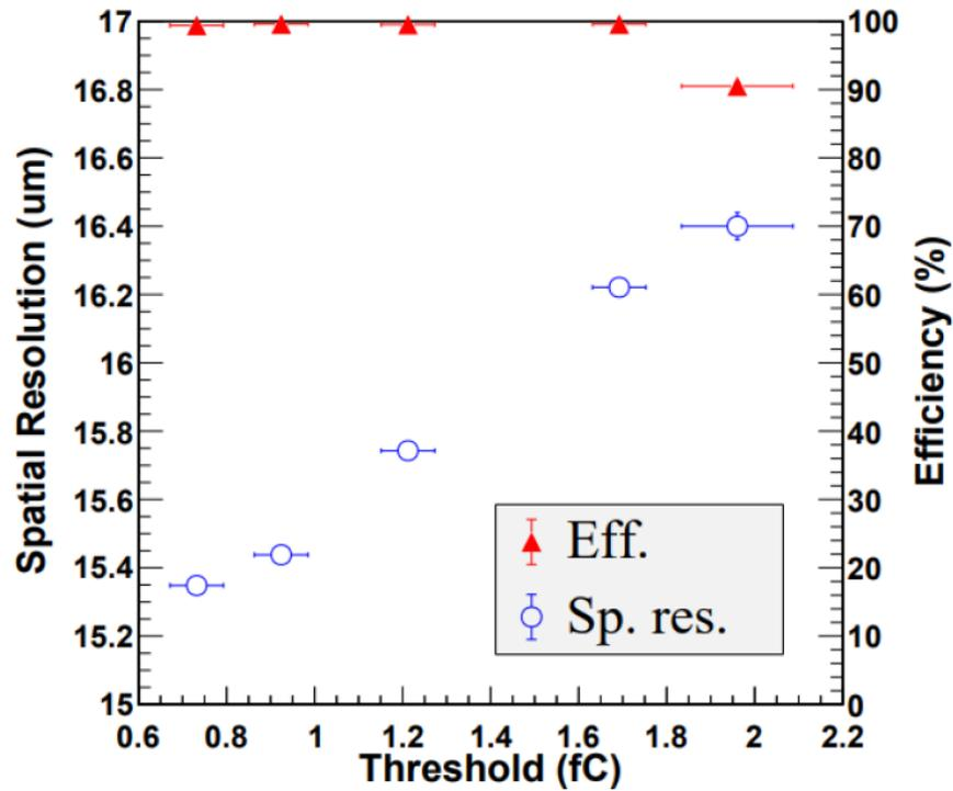
Spatial resolution and Efficiency vs ADC Threshold
