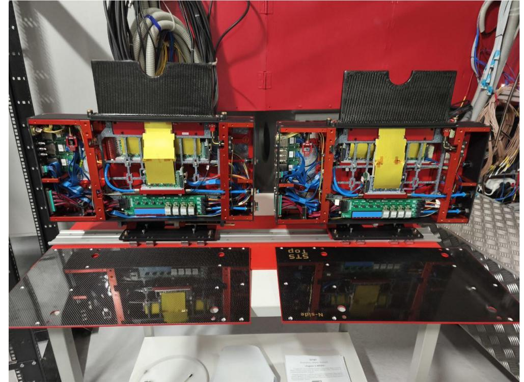
Two half-stations before installation inside the magnet
