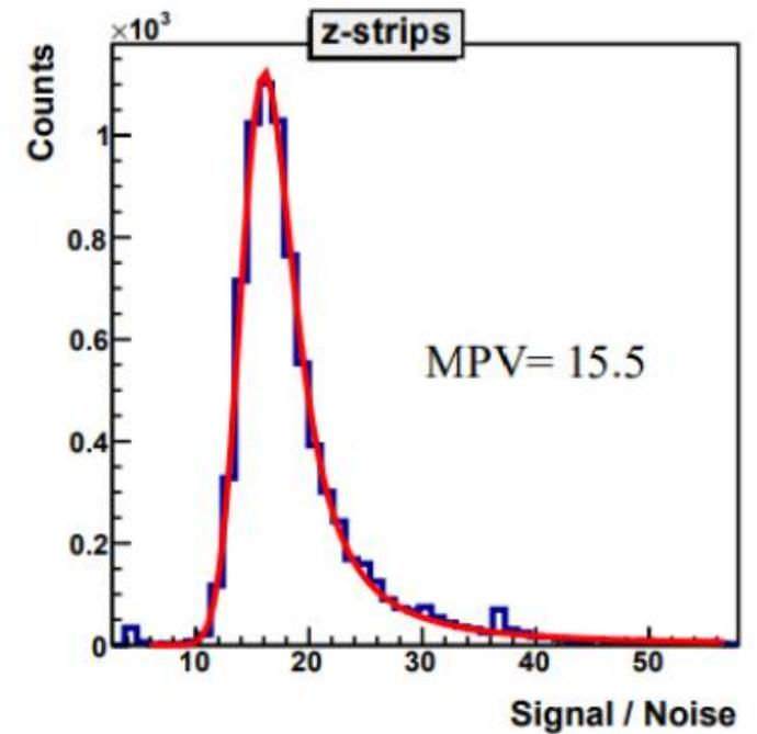
Signal-to-Noise distributions for the p-,n- and z-(with second metallization layer) strips for the 1 GeV protons
