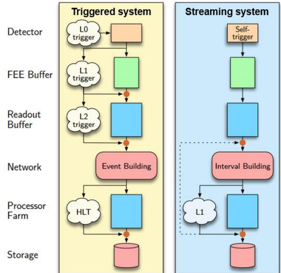
Comparison of triggered and free-streaming data acquisition systems
