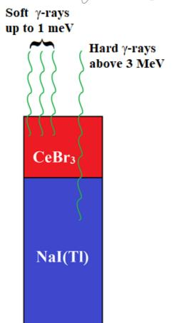
The phoswich detector technique allows avoiding the pile-up effect by separating the  $\gamma$ -quanta along their absorption length in the detector material.
