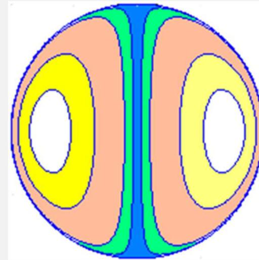
Hill showed that the incompressible Euler equations has a steady solution as a spherical vortex ring. The spherical vortex ring propagates without change of either velocity or shape.
