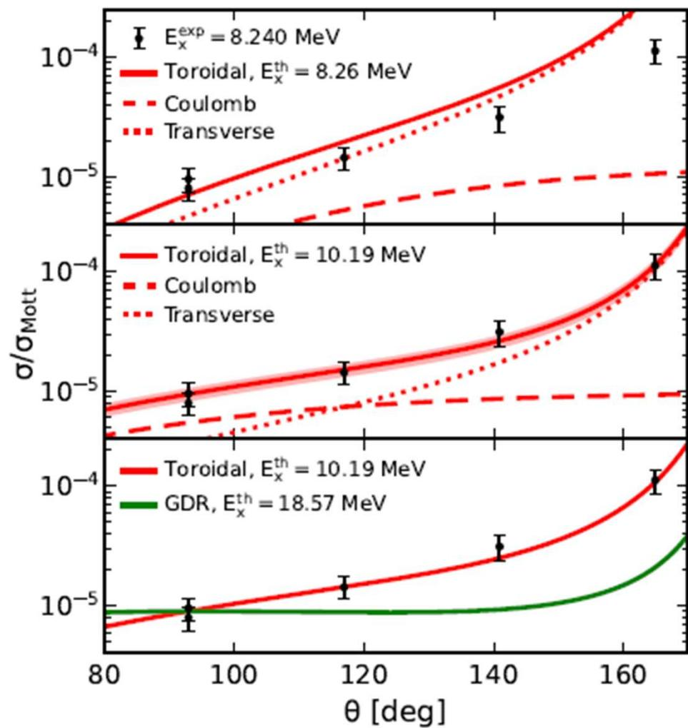
Electron scattering cross sections of the toroidal candidate at 8.240 MeV compared to QRPA predictions using the SV-mas10 interaction.
