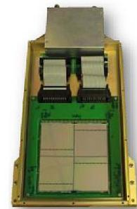
Each Si detector consists of 32x32 strips  $\sim 1.8$  mm thick
