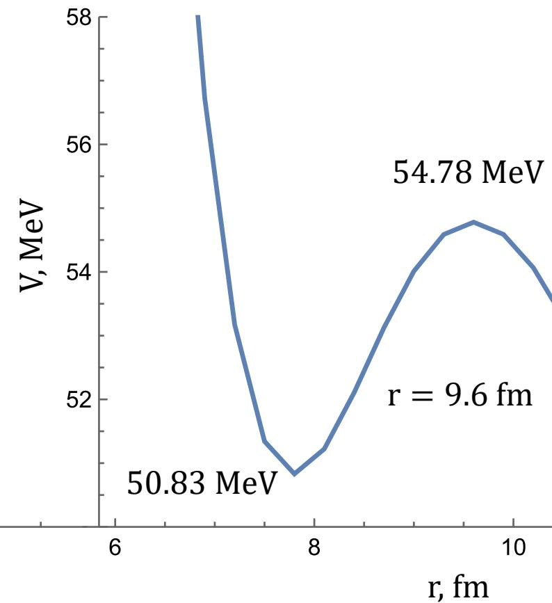
$r_{phen} = 10.58 \text{ fm}$ ,  $V_{phen} = 50.46 \text{ MeV}$   $^{48}\text{Ca} + ^{48}\text{Ca}$
