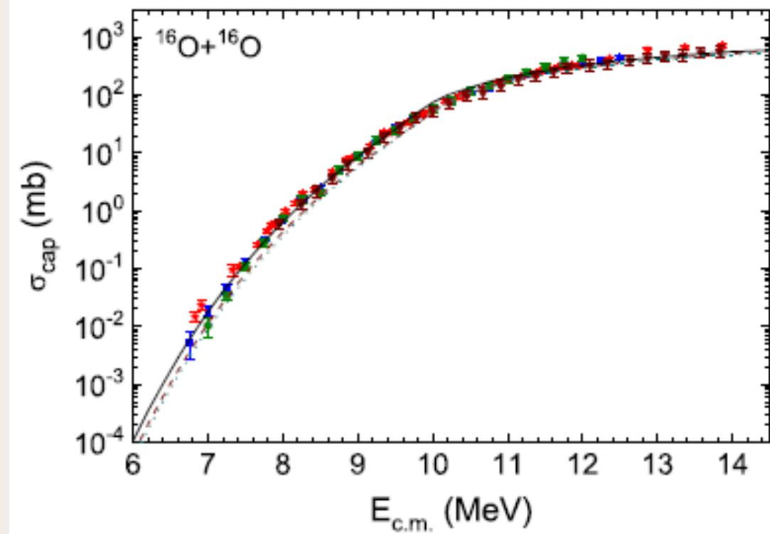
The fusion excitation functions calculated with phenomenologically adjusted (solid lines), self-consistent (dashed line), and parameterized (dotted line) potentials for the  $^{12}\text{C} + ^{12}\text{C}$  and  $^{16}\text{O} + ^{16}\text{O}$  reactions.
