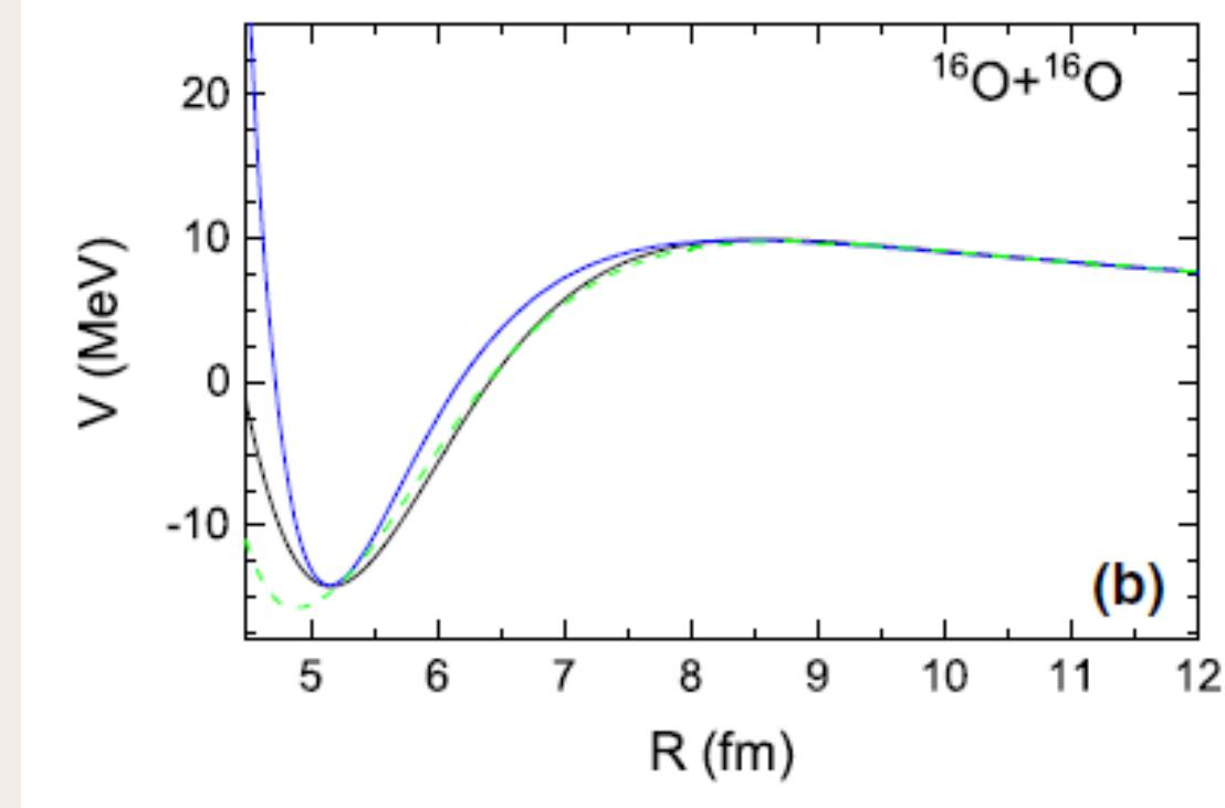
Comparison of nucleus-nucleus interaction potentials calculated with self-consistent (solid lines) and phenomenological (dashed lines) nucleon densities for the reactions  $^{40}\text{Ca} + ^{40}\text{Ca}$  and  $^{16}\text{O} + ^{16}\text{O}$ . The results of calculation with the parametrization of the nuclear part of the potential are shown by blue lines.
